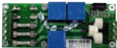
Power Measure PCB CIM 5, Repaired AS818511B
