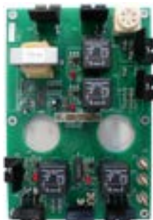
Relay Board mP-G, Repaired
