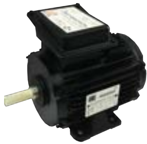
Evaporator Motor, Repaired
