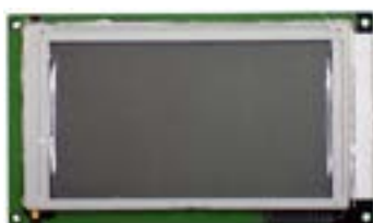
Display PCB CIM 5, Repaired AS818515A
