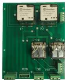
Relay Print, Repaired AT10501600
