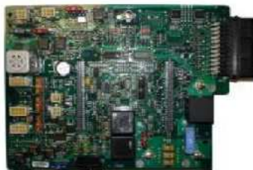
SR2 Interface Relay Board, Repaired
