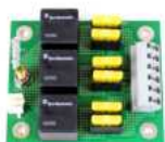
Relay Board Fan Control, Repaired
