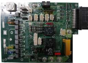
Spectrum TS Interface Relay Board, Repaired
