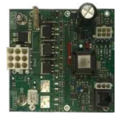
Logic Board Viento, Repaired AC12-00511-61 | AC12-00511-62 AC12-00511-64 | AC12-00511-67
