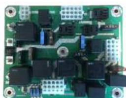
Relay Board Maxima, Repaired
