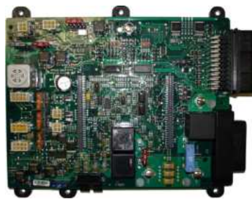
SR2 Controller & Interface Relay Board, Repaired
