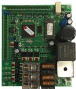
Microprocessor Control Unit, Repaired AT10501300
