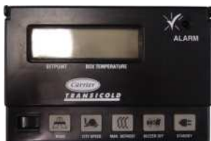
Cab Command Micro Control, Repaired AC12-00325-00 | AC12-00325-01 AC12-00325-02 P/N after repair AC12-00325-02
