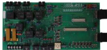
Relay Board Micro P-IV MT, Repaired AT41-1284 | AT41-2675 | AT41-2783 AT41-2784 | AT41-3054 | AT41-3055 AT41-3348 | AT41-3349 | AT41-3562 AT41-3563 | AT41-5763 | AT41-6931 AT41-7288 | AT41-7423
