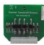
Diode Board, Repaired AC22-01102-XX
