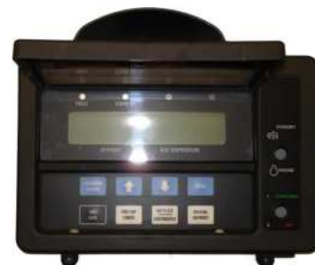
Display Board EasyCold, Repaired AC12-00515-00 (PCB Only) Display Assembly EasyCold, Repaired AC91-00333-00 | AC91-00333-03 P/N after repair AC91-00333-03
